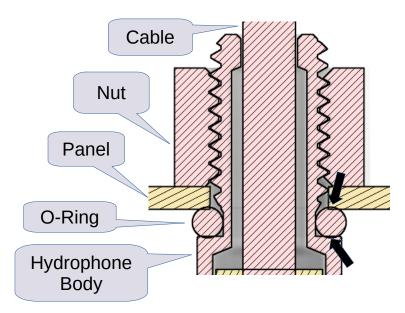
Straight 10mm hole through panel. Clamping force provides two points of contact for sealing (see arrows above). Positive pressure outside panel retains oring. Friction accommodates any common negative pressure. Sufficient for nearly all applications.
