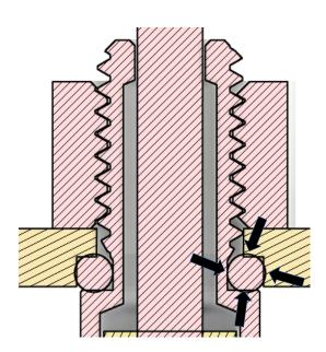
10mm hole with Ø12.5mm x 2mm deep counterbore provides four points of contact for sealing. O-ring fully retained against positive and negative pressure.
