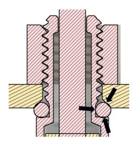
10mm hole with minimum 1mm chamfer provides three points of contact for sealing. O-ring fully retained against positive and negative pressure.
