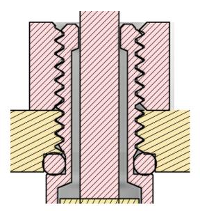
For high-pressure applications: Counterbore as at left, but panel is threaded with lock nut. Prevents crushing of o-ring under pressure and takes up play in thread for rigid mounting.
